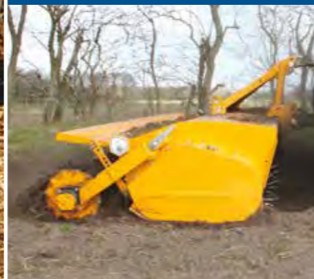
Rear crumbler To further break down soil structure.
