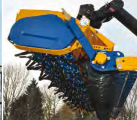
Dual rotors Two rotors connected via a single drive.
