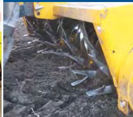
Front rotor Tines lift soil and turns into rear rotor to break down soil structure.
