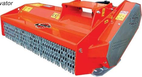
The TLBE-ST shredding head is perfect for crushing grass, canes and shrubs generally up to 7 cm, located near ditches, banks, and all sorts of very steep lands. It can be applied to excavator weighing from 5 tonnes and mainly to telescopic arms.
