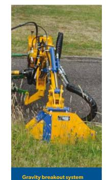
For protecting drive and machine during operation.
