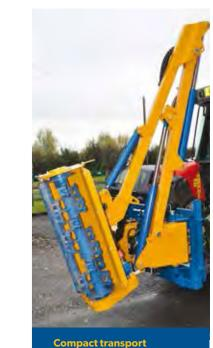
As a result of the 110° power slew the Osprey has a compact
